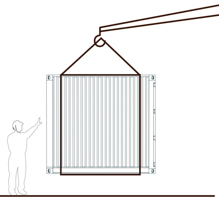
EXTERNAL DIMENSIONS 2850 (w) x 2440 (l) x 2600 (h) mm - INTERNAL DIMENSIONS 2640 (w) x 2300 (l) x 2250 (h) mm
